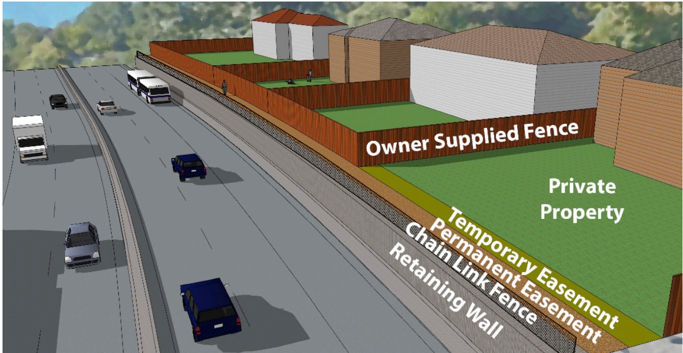
The Permanent Easement Proposed by Stride S3 Creates a No Man's Land, Between Fences
